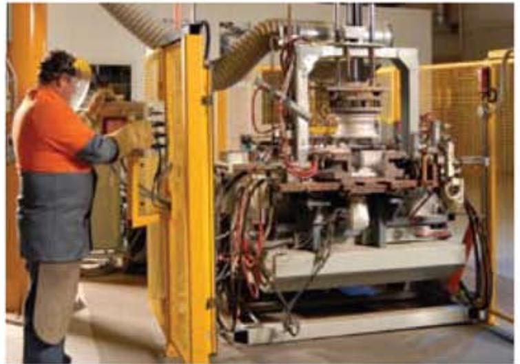
The pilot T-Mag™ machine, with 80-kg furnace capacity.
