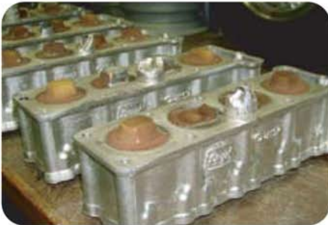
As-cast magnesium motorcycle engine blocks, showing small sprue and sand cores.
